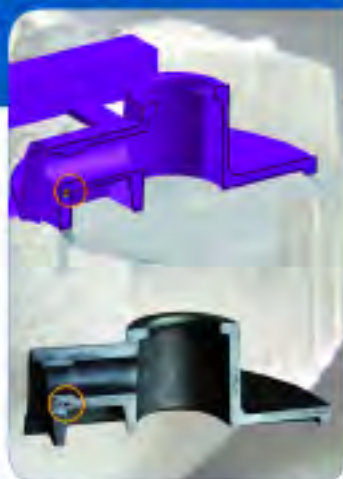
Predicted Shrinkage Porosity
